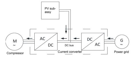
PV air conditioner and system power consumption working mode
