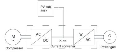
(single unit) Structure chart of PV direct-driven inverter VRF system
