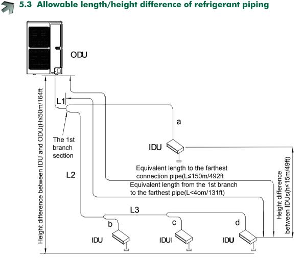
Each Y-type branch equals to 0.5m(1-5/8ft) and each branch header equals to 1.0m(3-1/4ft). **NOTICE!** The equivalent length of one Y shape branching joint is 0.5m(1-5/8ft). GMV-Y36WL/A-T(U)  $\$  GMV-Y48WL/A-T(U)  $\$  GMV-Y60WL/A-T(U):
