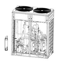
•Unscrew the support of the heat exchanging board, and remove the support and board.
