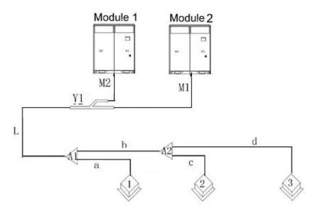
5.3 Select appropriate pipe between outdoor unit and the first indoor branch ("L") as per the pipe size of outdoor unit. Pipe size of basic outdoor module is shown as follows:
