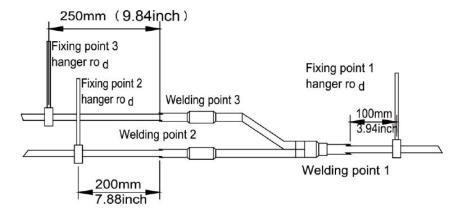
Branches of a manifold must be laid parallel and cannot be wrapped in superimposed mode.
