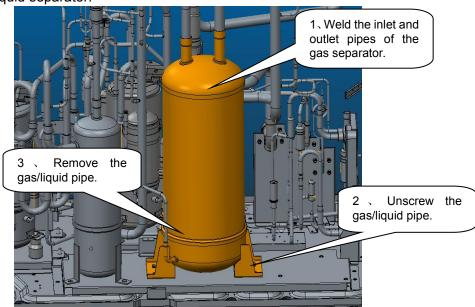
After the gas/liquid separator is taken out, check whether it contains impurities. The check procedure is as follows:
