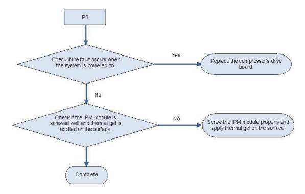
5) Recharging circuit faulty of the variable-frequency compressor drive board (ODU fault PF)
