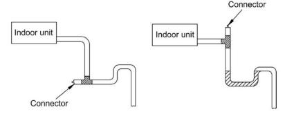
(5) During condensate water pipe installation, ensure a distance above 500mm (19.7inch) between the pipe and the electric box of the unit for maintenance. In a case when the space is not enough, the final piping way must be determined by the technical personnel.
