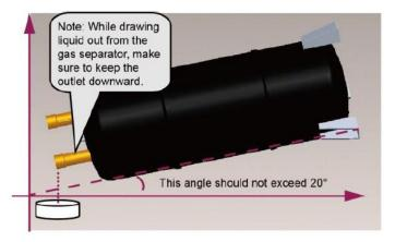
Use a glass container to hold the liquid. Check liquid impurities and colors and block the container for further factory inspection.
