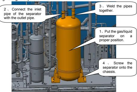
Step 9: Install a new oil separator.
