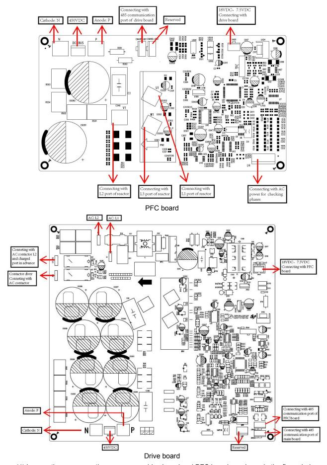
(4) Loosen the screws on the compressor drive board and PFC board, as shown in the figure below:
