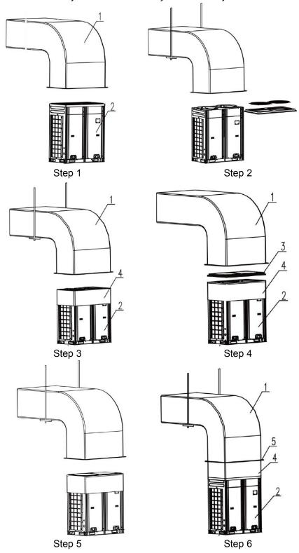
Method 2: Remove the unit top case. Detailed operations are as follows:
