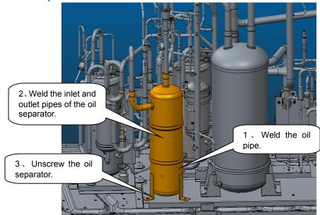
Remove the oil separator. For the removal procedure, refer to step 4. Tilt the separator to draw oil out into a container. Block the container for further factory inspection.
