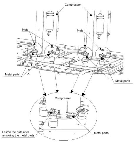
2) While installation, please make sure the metal parts are taken down. Then fasten the compressor fixed nuts again and re-wrap the soundproof material.
