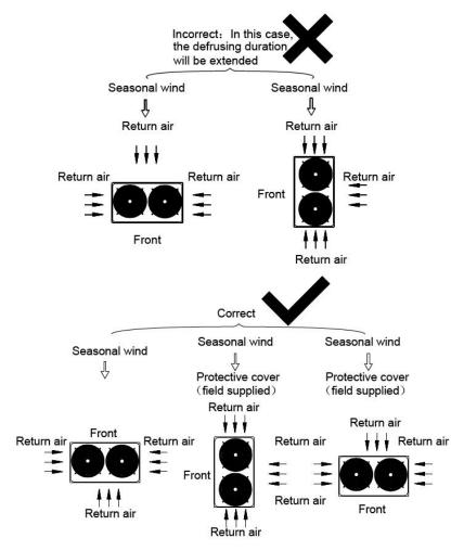
(5) Anti-monsoon installation requirements for unit connecting exhaust duct:
