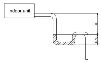
Install drain trap connectors as shown in the following figure.
