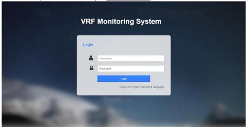
Step 3: Log in to VRF Monitoring System. For the first usage or after resetting the system, check equipment connection status in main interface (click "VRF monitoring system" on the left corner to enter the main interface), to make sure G module quantity and IDU & ODU quantity displayed on the page are consistent with actual quantity.
