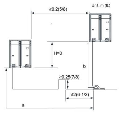
Note: when the distance between outdoor units exceeds 2m (6-1/2 feet), U-type oil trap should be added at low-pressure gas pipe.  $a \le 10m$  (32-7/8 feet);  $b \le 10m$  (32-7/8 feet).
