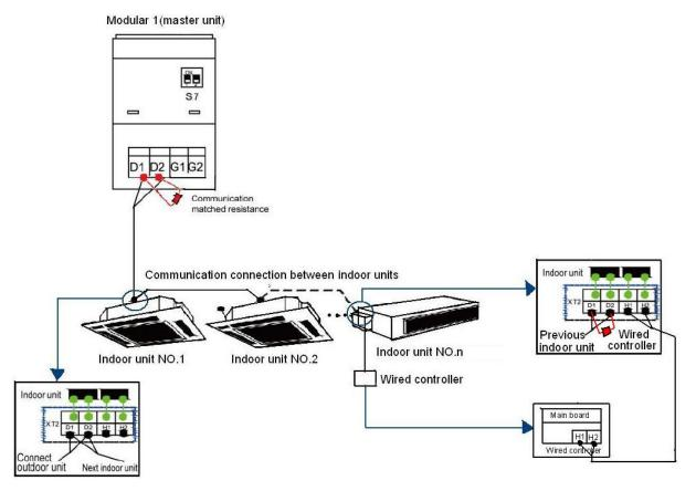
Connection of communication for multi-module system:
