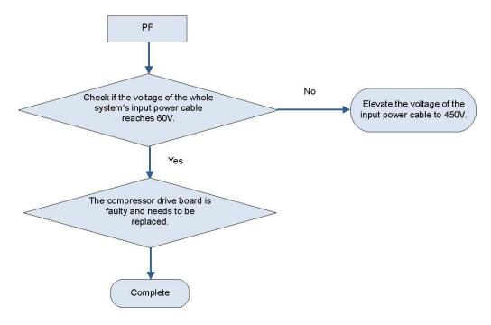
6) High voltage protection for the DC bus of the variable-frequency compressor's drive board (ODU fault PH)
