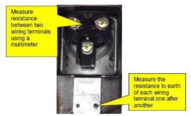
Measure the resistance to earth of each wiring terminal. The value should be 10 M $\Omega$ . If not, the compressor has an internal fault.
