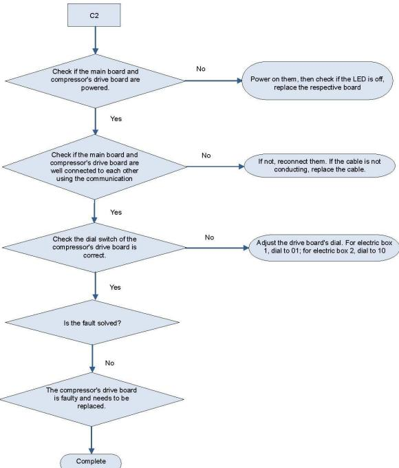
2) Faults in the current detection circuit drive of compressor (ODU fault PC) and out-of-step protection of compressor (ODU fault P9)
