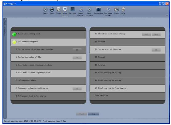
For the phase with "OK" displayed, a manual confirmation is required for entering the next commissioning step. Click "U" to display relevant information detected on this phase, which provides
