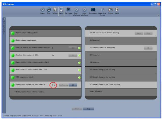
"indicates that commissioning is not passed on the phase and troubleshooting is required (after troubleshooting, the unit automatically enters the next step if no "OK" exists or click "OK" to enter the next step). Click "It to display relevant information detected on this phase, which provides references for troubleshooting. Click "Close" to close the information.
