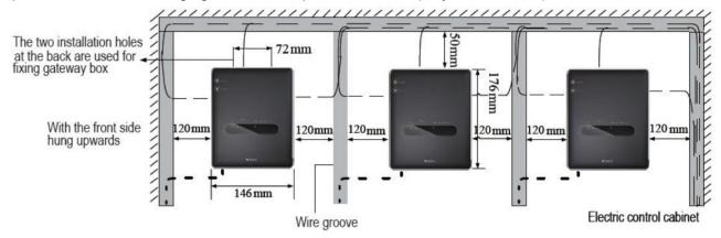
In the figure, slim dotted line is the communication wire and bold dotted line is the heavy current wire. The wiring way in the figure is only for reference.
