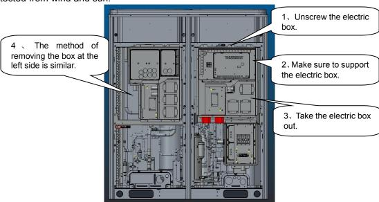
After the box is removed, take care with the removal of electric parts' lines. DO NOT pull the lines
