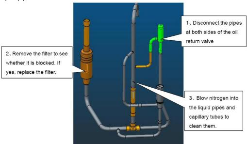
For other pipeline parts, clear them based on actual situation. If you do not replace the parts immediately, make sure to block the pipes with tapes, preventing air moistures and impurities from contaminating them.
