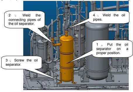
Step 10: Install a new compressor.
