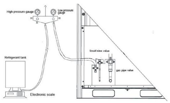
Step 2: Turn on the valves for the liquid and gas pipes of each module completely.
