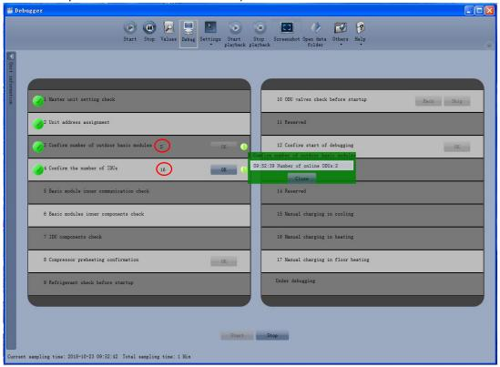
In the step "8 Compressor Preheat Confirmation", please confirm if the ODU valves are open manually at first, then confirm the compressor preheat time.
