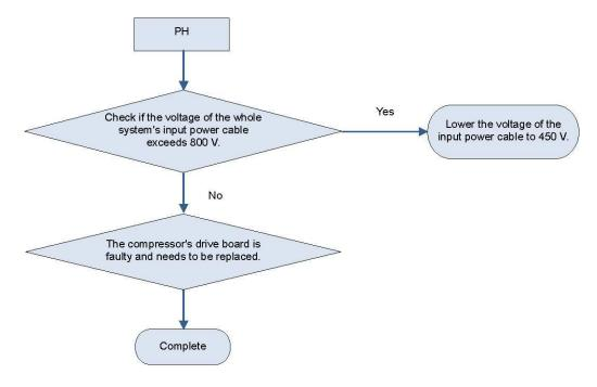
7) Low voltage protection for the DC bus of the variable-frequency compressor's drive board (ODU fault PL)
