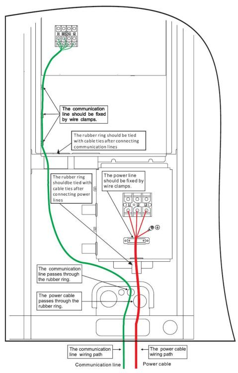
**NOTICE!** Provide a threading rubber ring when threading a strong power cable or a communication cable.
