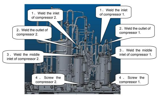
**Note:** Keep wiring identical to factory installation. Control varies with compressors. Wrong wiring or inverse connection of the compressors may cause damage to units.
