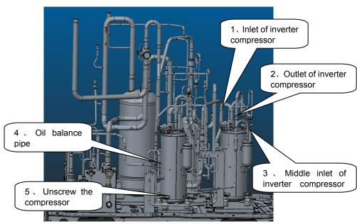
After the compressor and oil separator are removed, check oil quality. If oils are contaminated,
