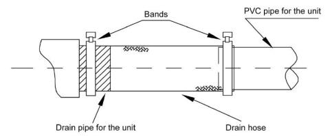
e. Apply insulation materials to the condensate water pipe joints to prevent dewing. d. Insulation for connection between the drain pipe and that of the IDU is shown in the following figure.
