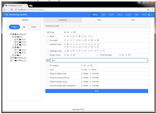
Note: The system provides timing control (daily, monthly and weekly), real-time failures, historical status data viewing and export, device group management and other functions.
