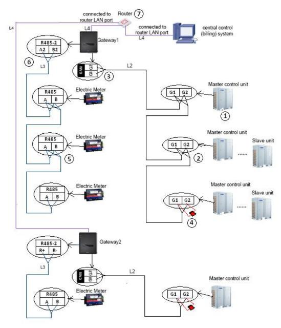
1) Communication wire connection between gateway and air conditioning master ODU:
