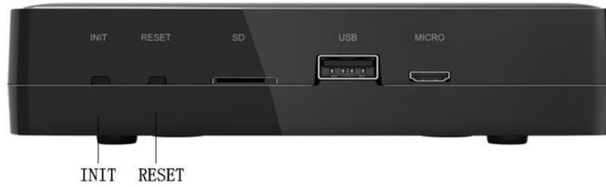
“INIT”: ex-factory settings restore button; hold on pressing it for 10s or hold on pressing it until eight communication indicators light on, then the system will restore ex-factory settings. Restoring ex-factory settings will clear all device information saved in the system, including IDU name, group name, IDU consumed electricity amount, etc. The system will restart automatically after clearing data.
