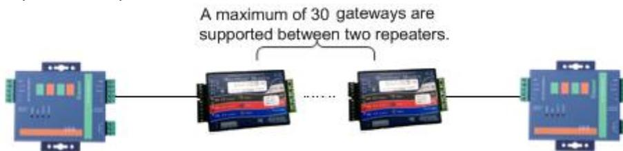
The total length of communication lines used between two repeaters cannot exceed 800 m.
