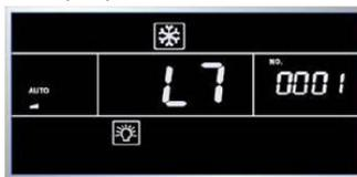
Method 1: If the IDU is configured with wired control, stop the IDU (except for lock mode) and press and hold the “MODE” button for 5 seconds to enter setting mode. After setting, the “Master” icon will be highlighted and the wired control buzzer will beep once.
