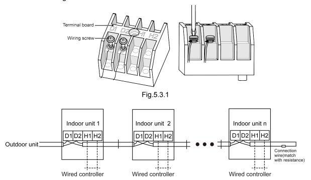
**NOTICE** Indoor unit quantity n is according to the outdoor unit capacity.
