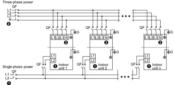
**NOTICE** (1) Connect wires for single-phase unit according to figure **1** and connect wires for three-phase unit according to figure **2**.
