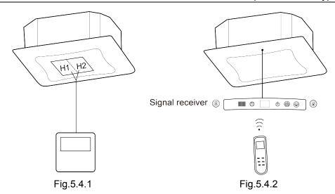
2) Both IDU and wired controller are equipped with signal receiver, and available for wireless control respectively.
