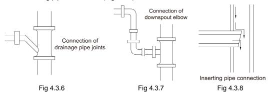
(9) Drain pipes should have a downward slope of at least 1%~2%, in order to prevent pipes from sagging, install hanger bracket at intervals of 1000~1500mm (39-3/8~59in.).
