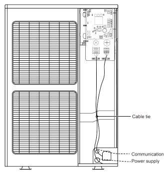
Fig. 4.6.4 Engineering Wiring View
