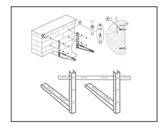
Make sure the chosen installation location meets with specified requirements and wall design and construction is suitable and strong enough to hold the brackets and the associated equipment loads. Anchors and related mounting hardware are provided.
